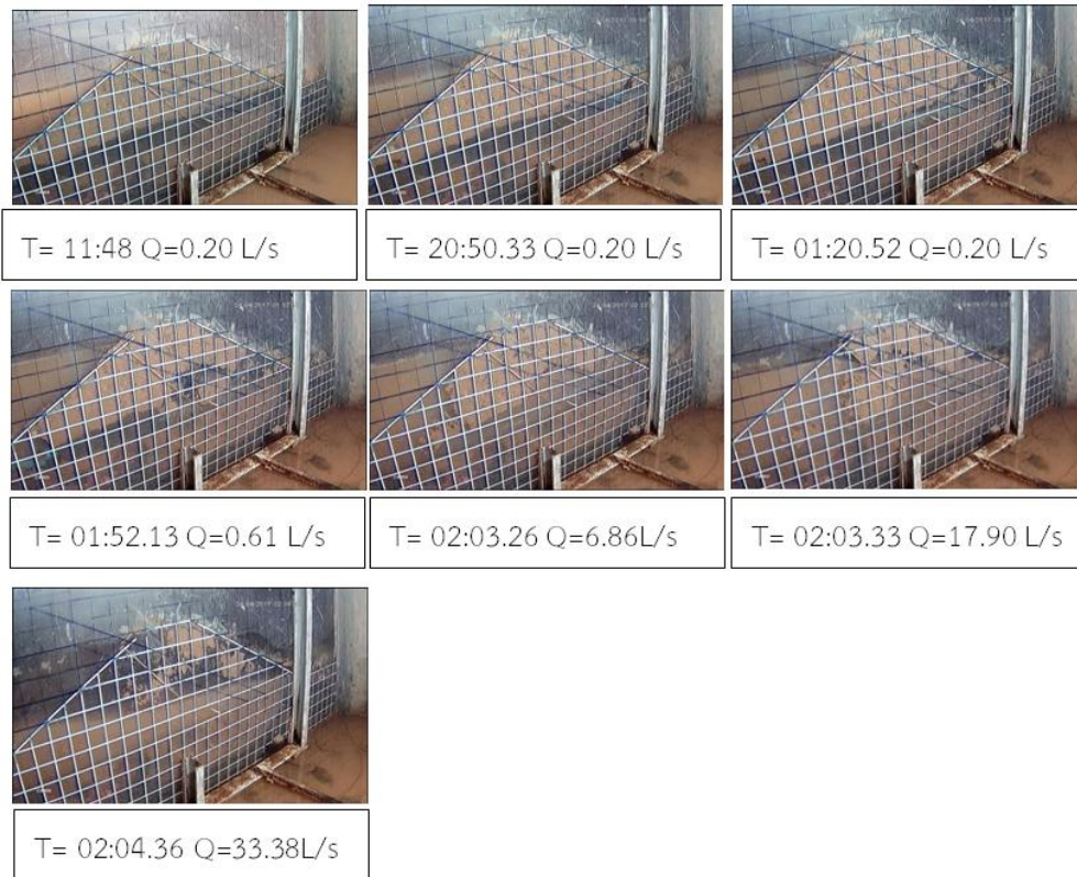
Figure 9 Internal erosion of embankment when pipe culvert near solid wall
